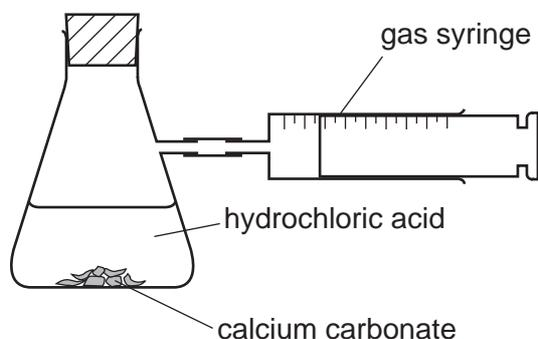
The time to collect  $50\text{ cm}^3$  of gas is measured.
